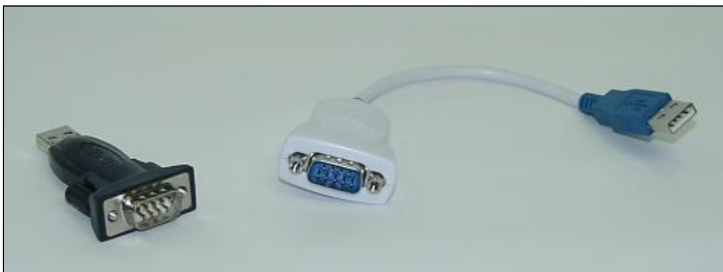
Figure 2-4. USB-to-Serial Converters using the FTDI Chipset.
