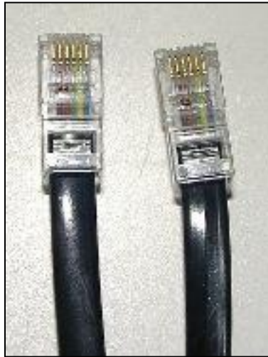
Figure 2-3. Close up of Reverse Cable Plugs – note each end is wired identically.
