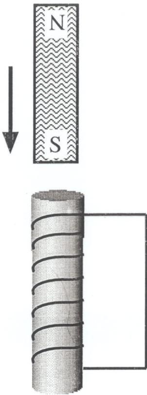
The south pole of a bar magnet is approaching the solenoid
