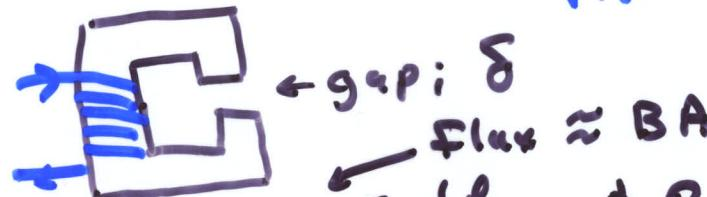
$$\oint \vec{H} \cdot d\vec{l} = NI = \oint \frac{\vec{B}}{\mu} \cdot d\vec{l} = \phi \int \frac{dl}{\mu A} = \phi R_{\text{tot}}$$
