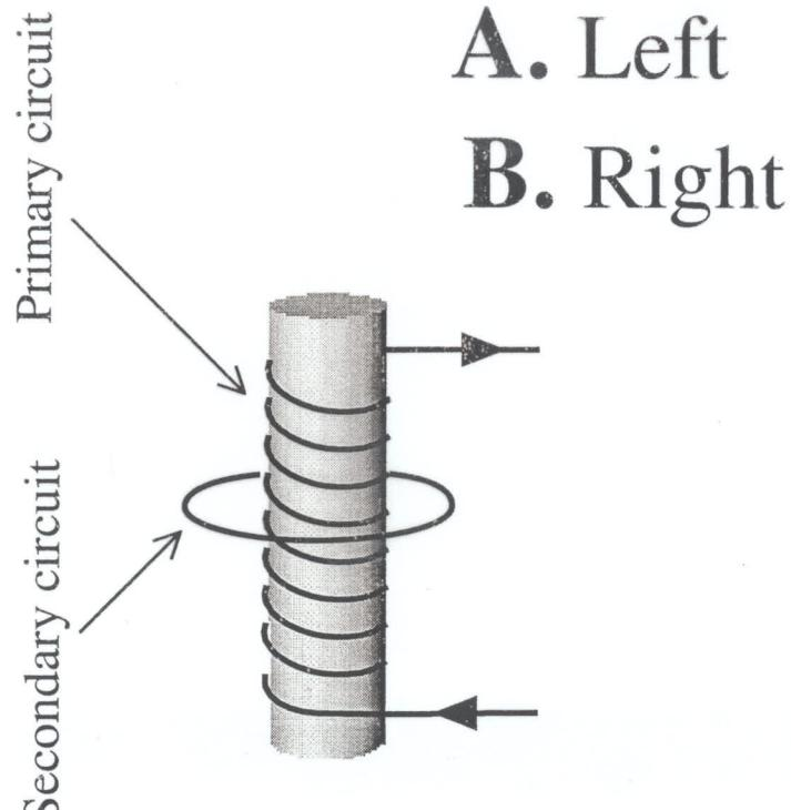
The current shown flowing through the primary circuit is increasing
