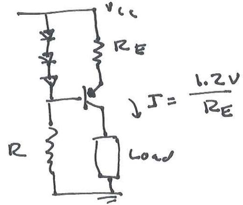
Early Effect ( $10^{-4} = h_{re}$ )  $\rightarrow$   $V_{CE}$  affects the on voltage of BE diode.
