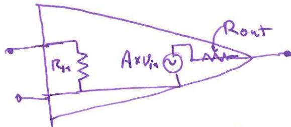
Remarks: it turns out that  $R_{in} \rightarrow \infty$  &  $R_{out} \rightarrow 0$  are good characteristics of amp.
