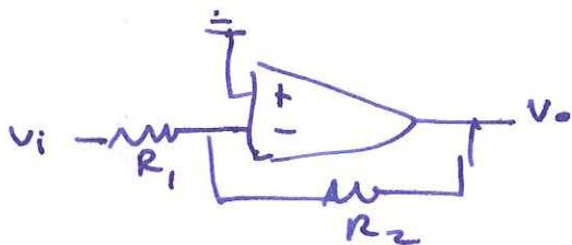
$$\frac{V_+ - V_-}{R_1} = \frac{V_- - V_o}{R_2}$$
