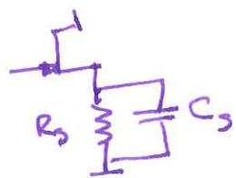
Select  $R_s \Rightarrow I_D R_s = \text{desired } |V_{GS}|$
