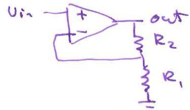
$$A(V_{in} - BV_{out}) = V_{out}$$
