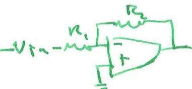
in both cases an addition current flow of  $\frac{V}{R_1 + R_2}$  happens - i.e. must add this current to above
