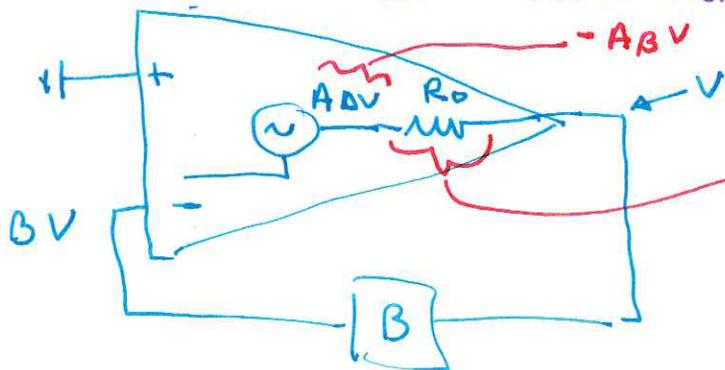
$$\text{voltage drop} = V - -ABV = (1 + AB)V$$
