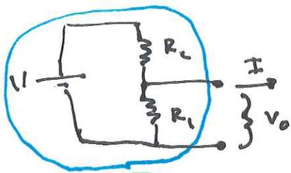
$$V_0 = \frac{R_L}{R_1 + R_L} V - R_1 \parallel R_L I$$
