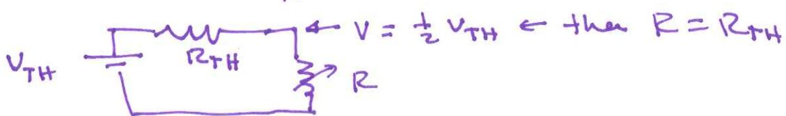
Or just attach any  $R$  and measure the resulting "voltage drop"  $\Delta V$ , then  $R_{TH} = \frac{R}{\frac{V_{TH}}{\Delta V} - 1}$
