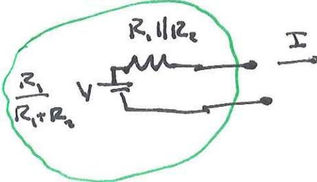
$$V_0 = \frac{R_L}{R_1 + R_L} V - R_1 \parallel R_L I$$
