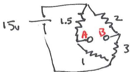
$$\left. \begin{aligned} V_A &= \frac{1}{2.5} 15 = 6V \\ V_B &= \frac{3}{5} 15 = 9V \end{aligned} \right\} U_{TH} = 3V$$
