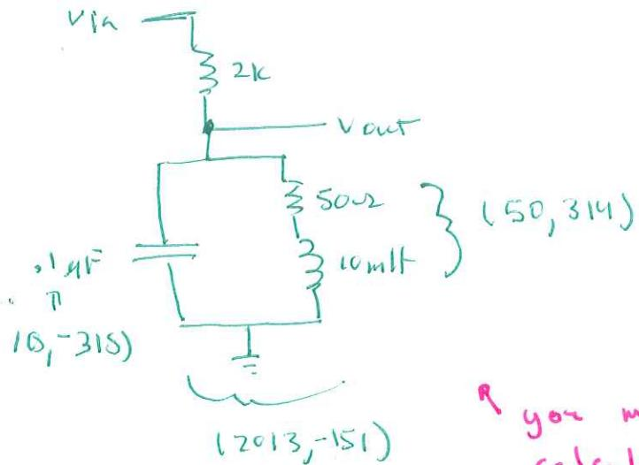
$$\frac{V_{out}}{V_{in}} = \frac{(2013, -151)}{2000 + (2013, -151)}$$
