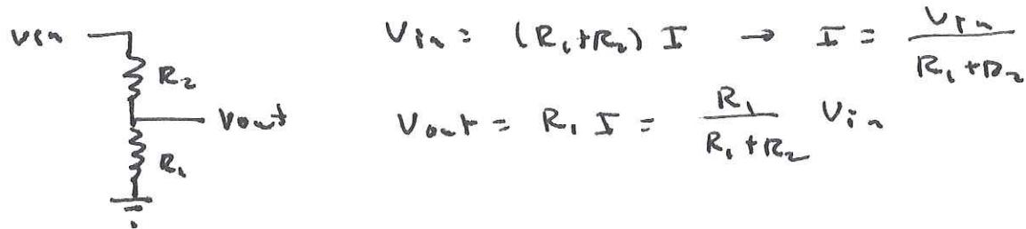
Q: the above assumed current thru  $R_2$  = current thru  $R_1$ , what if some current is drawn out -
