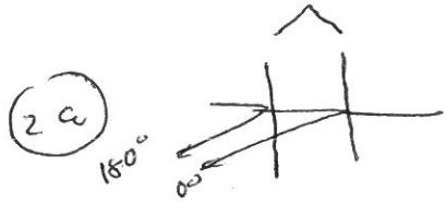
$$2t = (n + \frac{1}{2}) \frac{\lambda}{n} \leftarrow \begin{matrix} \text{integer} \\ \text{index of refraction} \end{matrix}$$
