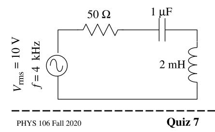
(A) Calculate the reactance of components: C and L. (B) Calculate the total impedance of the circuit. (C) Calculate the rms current flowing. (D) Calculate the rms voltage drop across R.
