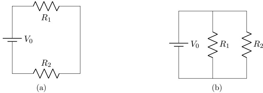
Figure 4.2: Two resistors connected (a) in series and (b) in parallel with a power supply.
