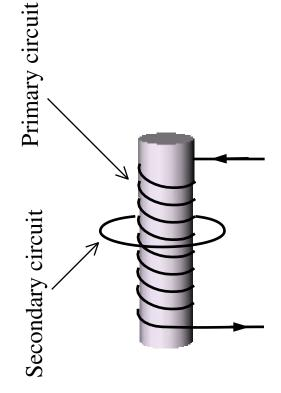
For several minutes no current has been flowing through the primary circuit. A current now starts and increases in the direction indicated. Place an arrow on the front surface of the secondary circuit showing the direction of any resulting current induced in the secondary circuit
