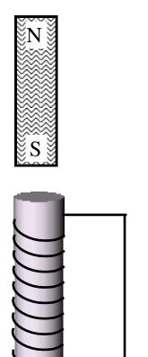
The south pole of a bar magnet has been sitting away from the end of a solenoid. The bar magnet is now moved vertically towards the solenoid. Place an arrow on the solenoid's vertical connecting wire showing the direction of any resulting current induced in the solenoid.
